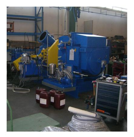
Horizontal Francis Configuration permitts to easily insert a flywheel for connection to a Stand Alone Grid.
